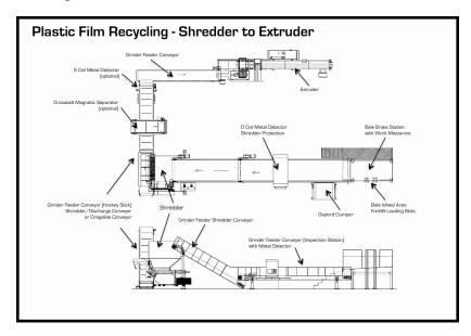
Recycling systems of this type call for a metal detection inspection conveyor to examine
