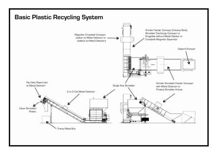
contaminated with metal can damage shredder and grinder knives.
